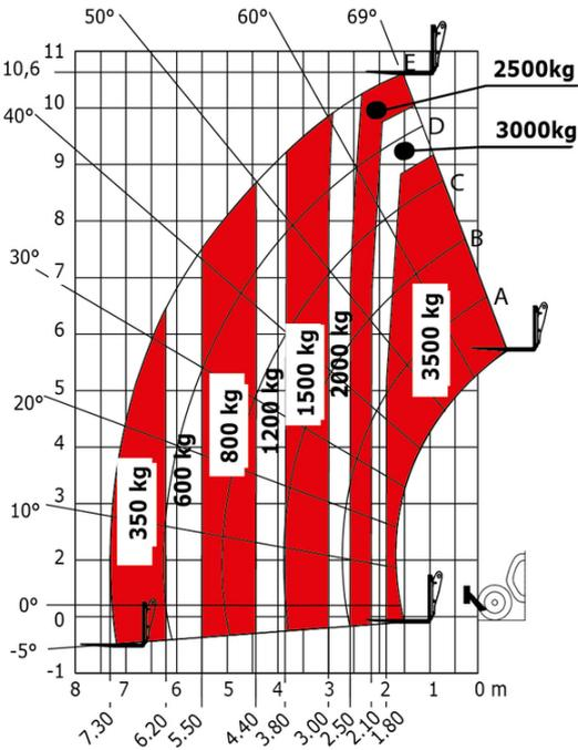
Machine on lowered stabilisers with forks Metric
