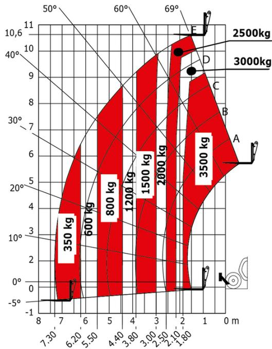
Machine on lowered stabilisers with forks Metric
