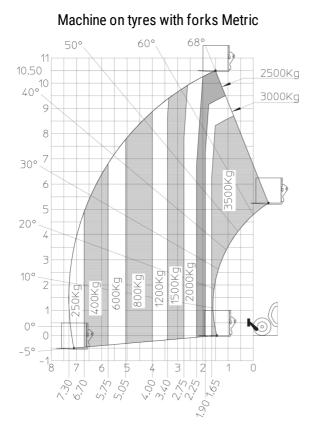
Machine on lowered stabilisers with forks Metric
