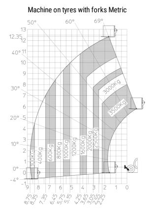
Machine on lowered stabilisers with forks Metric
