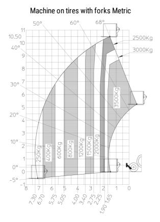
Machine on lowered stabilisers with forks Metric
