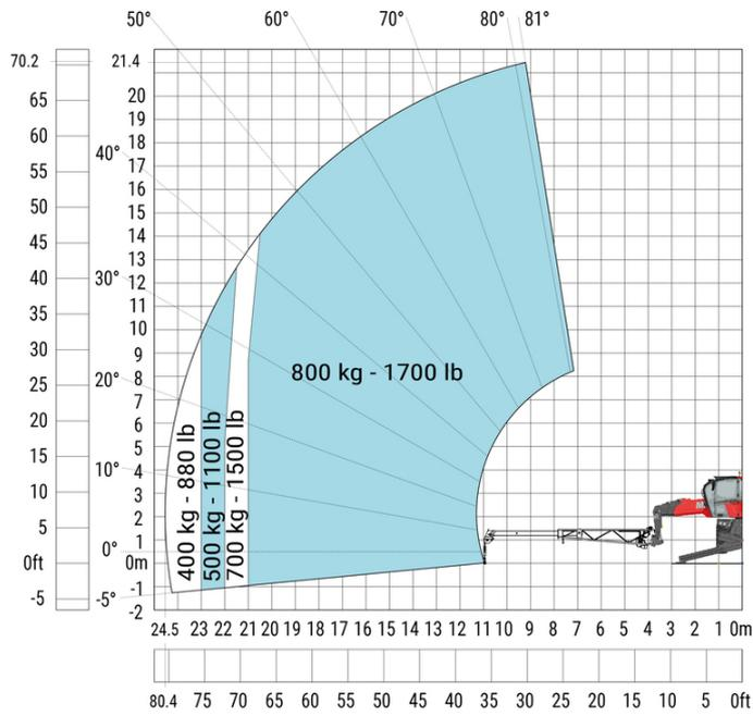
Machine on lowered stabilisers with hook 6000 kg (Imperial)
