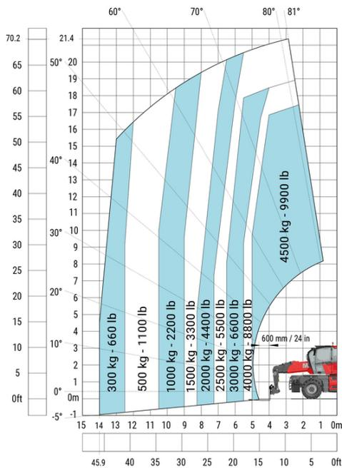
Machine on lowered stabilizers with forks (CAF) Imperial
