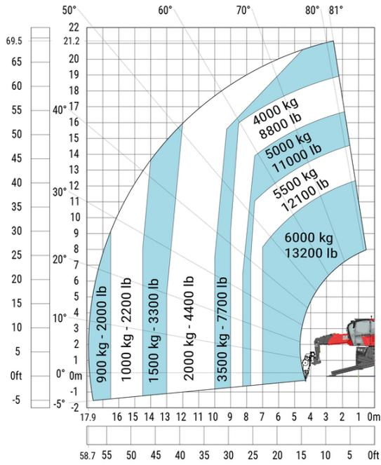
Machine on lowered stabilisers with 1500 kg jib with winch (Imperial)
