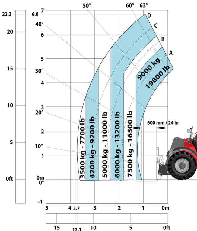
Machine on tires with winch 9000 kg (Imperial)
