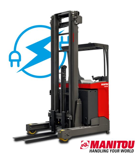
MANITOU ER 20 HD Electrical Seated 2000 kg 600 mm 416 mm 1530 mm 4150 kg Vulkollan 0 x 355 x 155 2 x 285\*105 1/2 0 mm 1128 mm 2205 mm 1077 mm 2485 mm 1335 mm 1270 mm 40 mm x 100 mm / 1150 mm 2A 903 mm 316 mm / 697 mm 70 mm 2788 mm 2831 mm 1750 mm 14.30 km/h / 14.50 km/h 0.37 m/s / 0.63 m/s 0.55 m/s / 0.43 m/s 0.20 m/s / 0.20 m/s 6.30 % / 9.40 % Electric 7.20 kW 15 kW DIN 43531 C 48 V / 620 Ah 920 kg Electronic 25 l/min 60.80 dB
