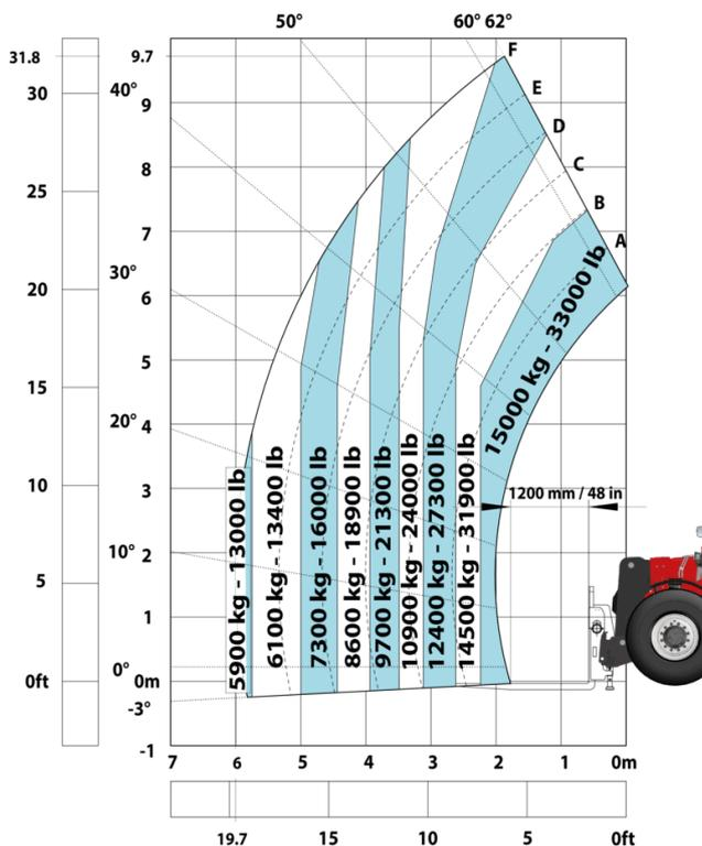
Machine on tires with winch 20000 kg (Metric)
