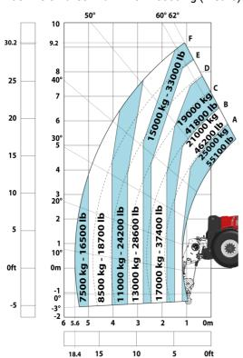
Machine on tires with 3-hook jib 25000 kg (Metric)
