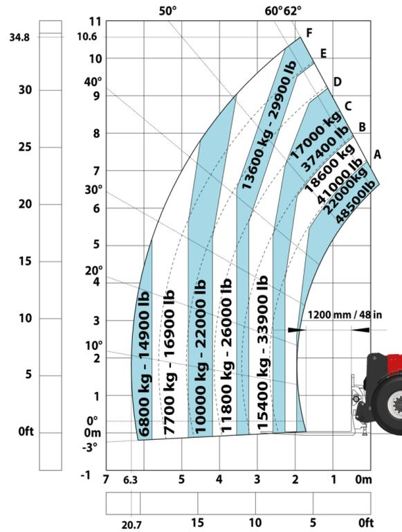
Machine on tires with winch 25000 kg (Metric)
