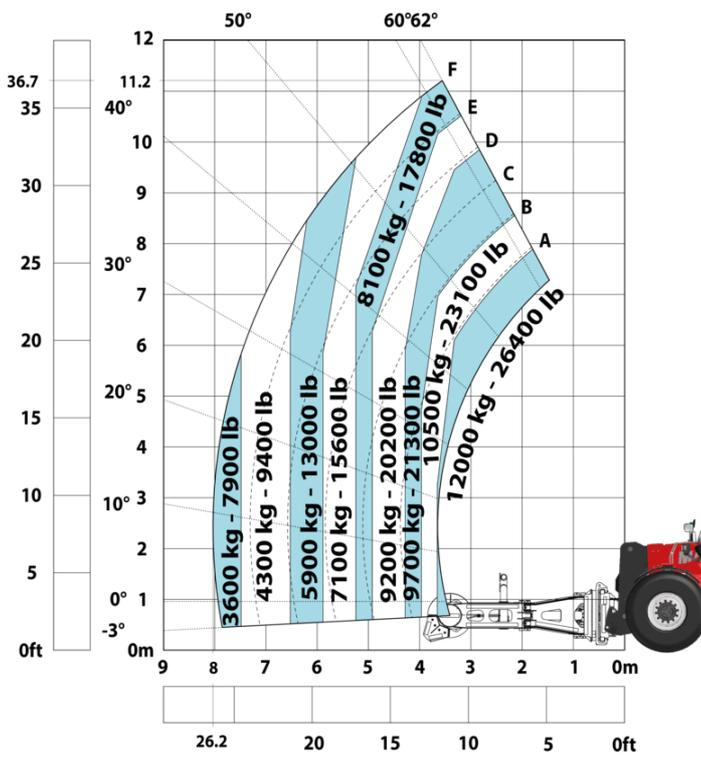
Machine on tires with cylinder handler CH 10 (Metric)
