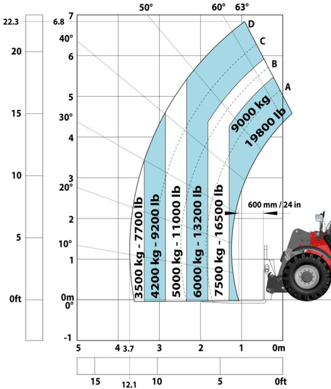
Machine on tires with winch 9000 kg (Metric)
