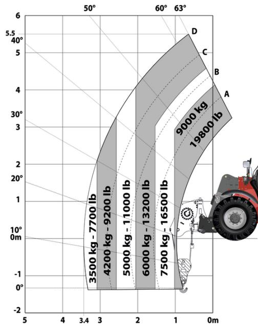
Machine on tires with 3-hook jib 9000 kg (Metric)
