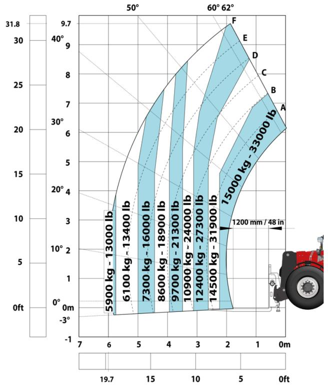
Machine on tires with winch 20000 kg (Metric)
