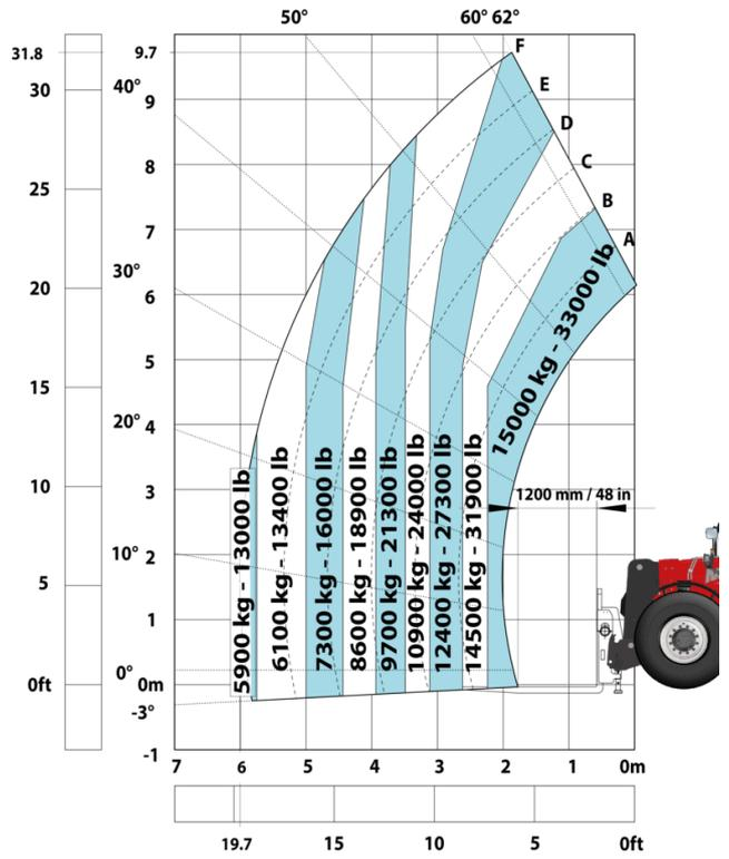
Machine on tires with winch 20000 kg (Imperial)
