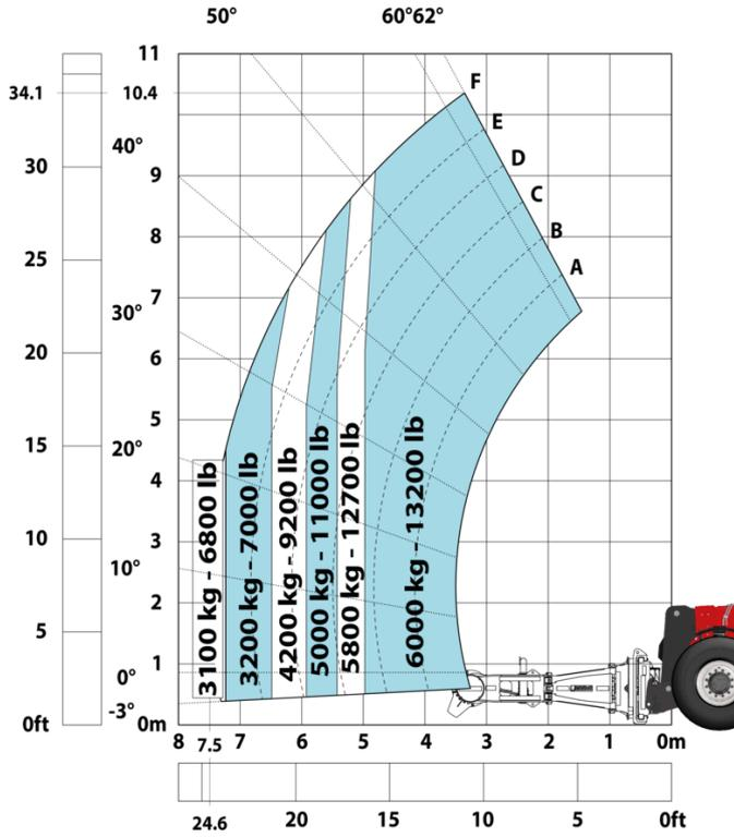
Machine on tires with cylinder handler CH 10 (Imperial)
