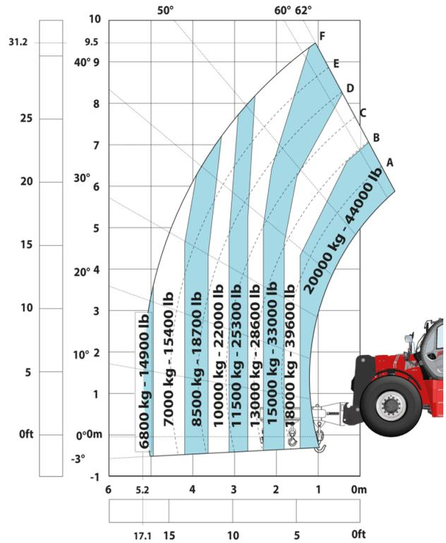
Machine on tyres with tyre handler TH 57 (Metric)
