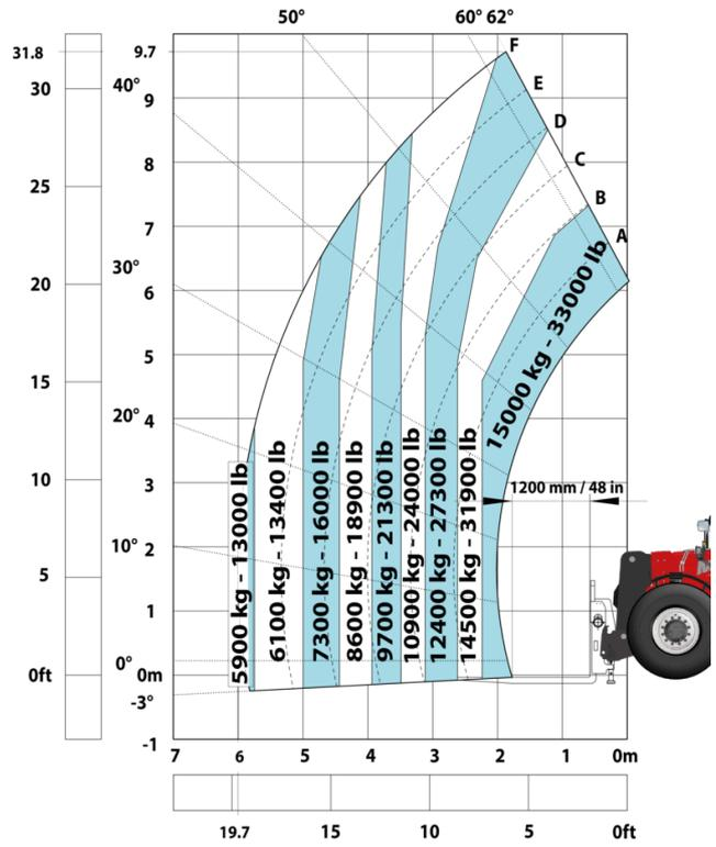
Machine on tyres with winch 20000 kg (Metric)
