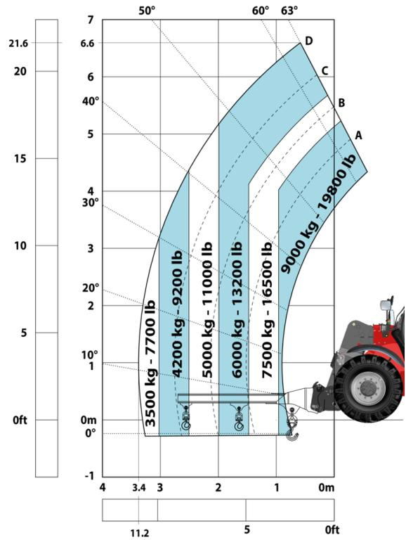
Machine on tires with platform Metric
