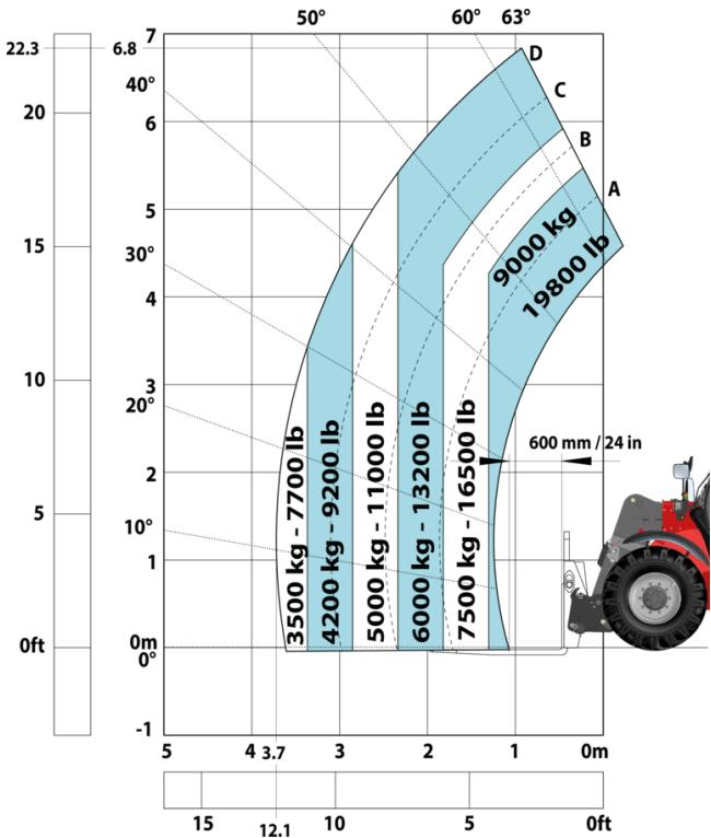
Machine on tires with 3-hook jib 9000 kg (Metric)
