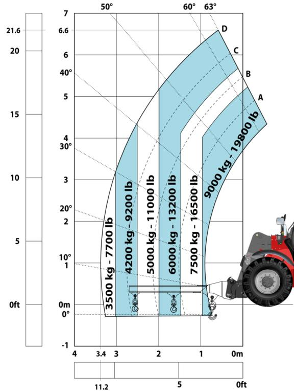
Machine on tires with platform Metric
