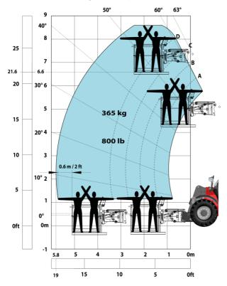
Machine on tyres with 3-hook jib 9000 kg (Metric)
