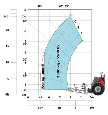
Machine on tyres with cylinder handler CH 4 (Metric)
