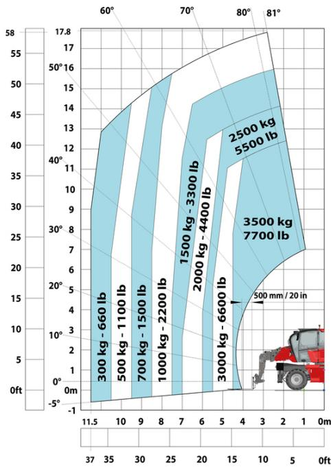
Machine on lowered stabilisers with forks Metric
