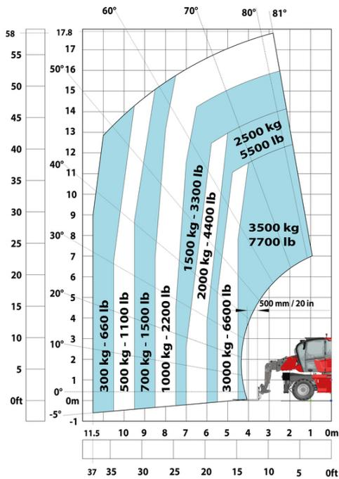
Machine on lowered stabilisers with forks Metric
