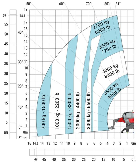
Machine on lowered stabilisers with 365 kg platform Metric Machine on lowered stabilisers with 1000 kg platform
