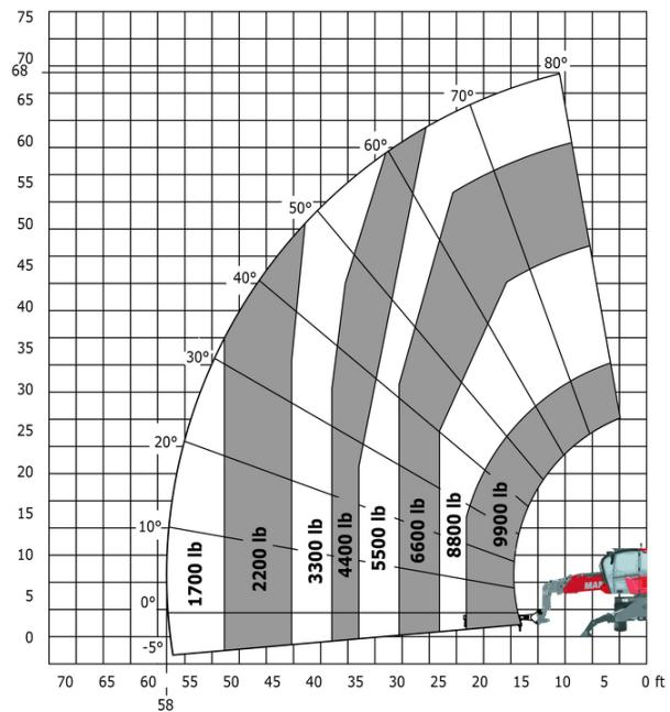
Machine on lowered stabilisers with 365 kg platform
