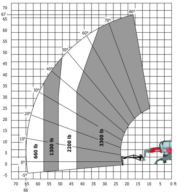
Machine on lowered stabilisers with hook 5000 kg (Imperial)
