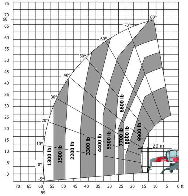
Machine on lowered stabilisers with winch 5000 kg Imperial Machine on lowered stabilisers with 4000 kg jib (Imperial)
