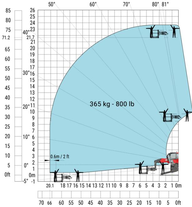
Machine on lowered stabilisers with 1000 kg platform Imperial
