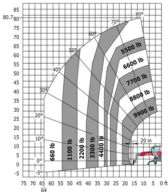
Machine on lowered stabilisers with winch 5000 kg Imperial Machine on lowered stabilisers with 4000 kg jib (Imperial)
