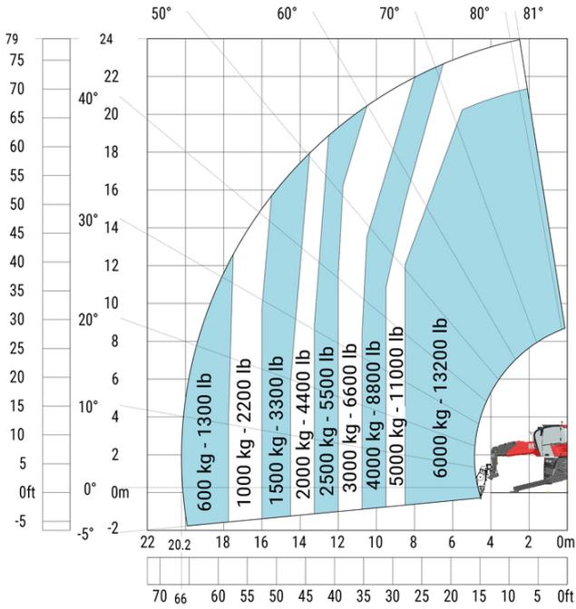
Machine on lowered stabilisers with winch 7200 kg (Imperial)
