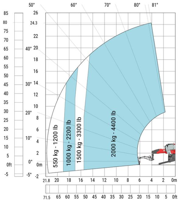
Machine on lowered stabilisers with extensible jib with winch (Imperial)
