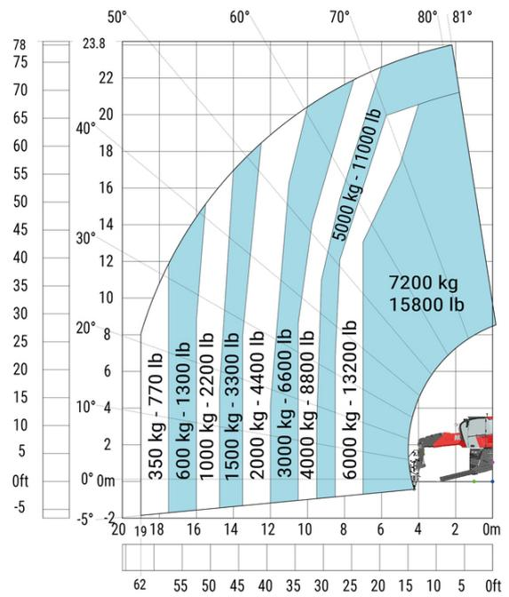
Machine on lowered stabilisers with 1500 kg jib Imperial
