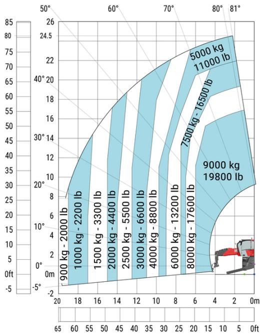
Machine on lowered stabilisers with 1000 kg platform Imperial
