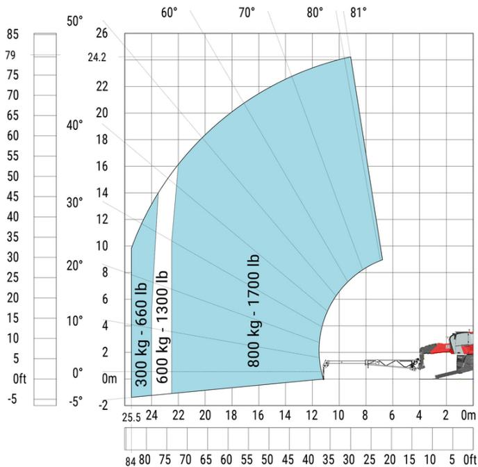
Machine on lowered stabilisers with hook 9000 kg (Imperial)
