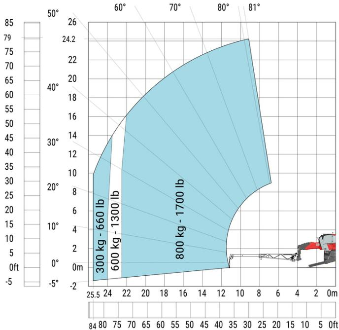
Machine on lowered stabilisers with hook 9000 kg (Metric)
