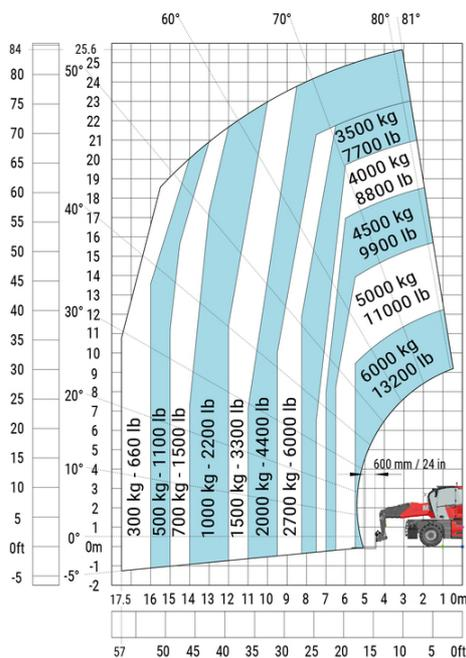
Machine on lowered stabilisers with forks (CAF) Metric
