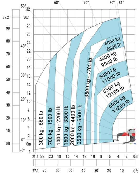
Machine on lowered stabilisers with 2000 kg jib with winch (Metric)    Machine on lowered stabilisers with 365 kg platform Metric
