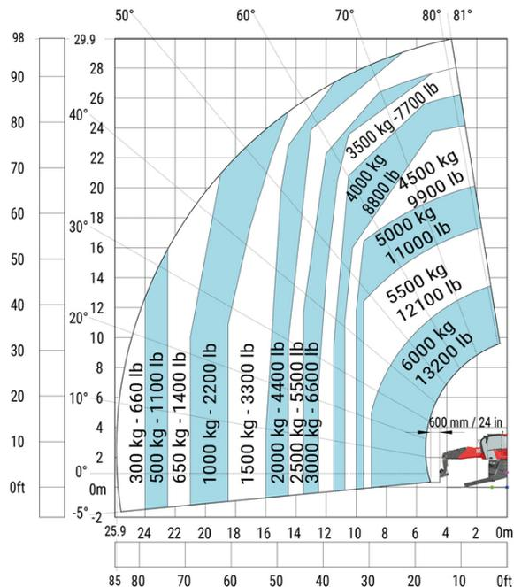
Machine on lowered stabilisers with winch 6000 kg (Metric)    Machine on lowered stabilisers with 6000 kg jib (Metric)
