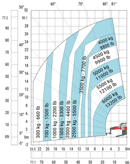
Machine on lowered stabilisers with 2000 kg jib with winch (Imperial)
