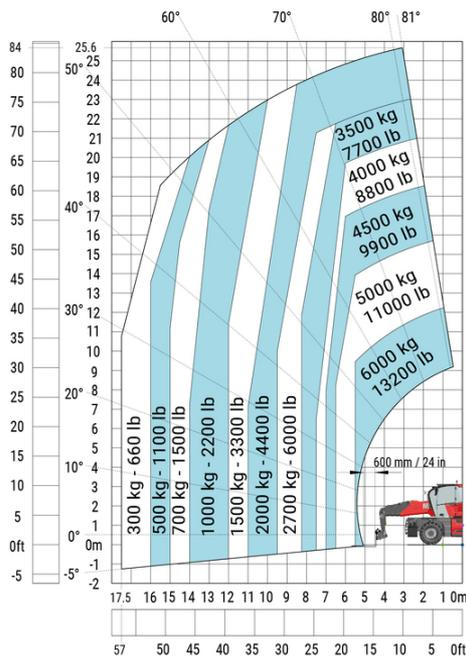
Machine on lowered stabilisers with forks (CAF) Imperial
