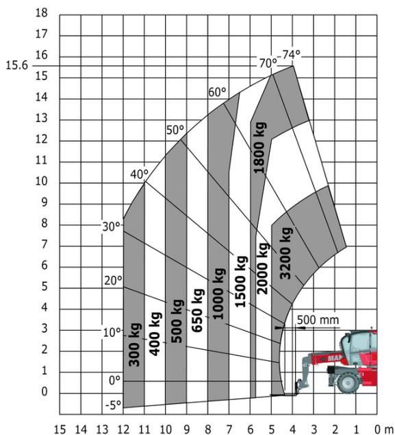
Machine on lowered stabilisers with forks Metric
