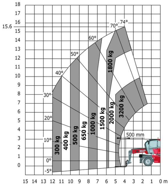
Machine on lowered stabilisers with forks Metric
