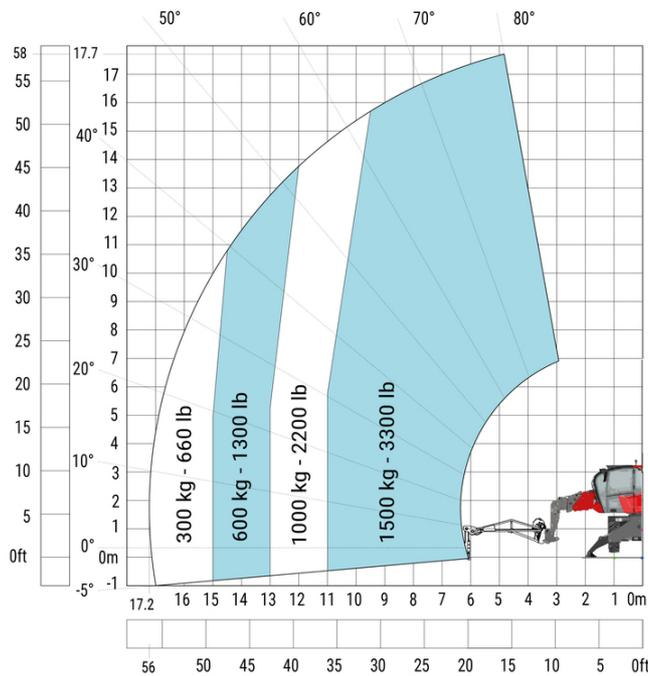
Machine on lowered stabilisers with hook 5000 kg (Metric) Machine on lowered stabilisers with 365 kg platform Metric
