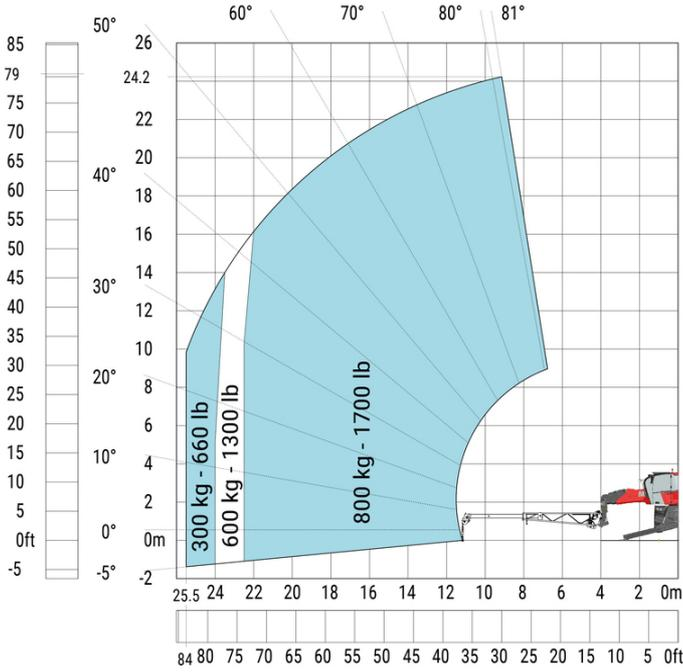
Machine on lowered stabilisers with hook 9000 kg (Metric)
