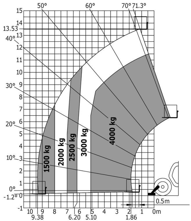
Machine on stabilisers with Man basket Metric
