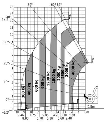
Machine on lowered stabilisers with forks Metric
