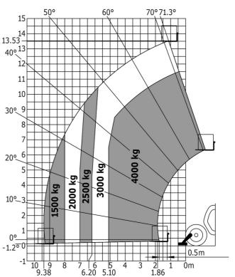
Machine on stabilisers with Man basket Metric
