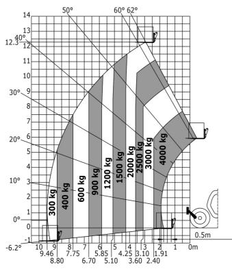
Machine on lowered stabilisers with forks Metric
