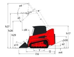
Met 1043.26 kg 1490.50 kg 1088.62 kg 4196 kg 3817 kg 4196 kg 4026 mm 3073 mm 2045 mm 42 ° 2300 mm 3589 mm 927 mm 92 ° 965 mm 1753 mm 191 mm 2789 mm 2235 mm 1374 mm 1625 mm 15.30 km/h 10.30 km/h Hydrostatic Yanmar 4TNV98CT-XNGL Stage V, Tier 4 53.70 kW 52.70 kW 294 Nm / 1800 rpm Diesel 4 72 Hp Water 12 V 100 A 3 kW 86.50 l/min 239.59 bar 114 l/min 229.25 bar 148.80 l 3.30 I 18 I
