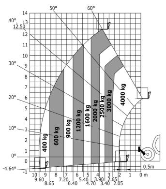
Machine on lowered stabilisers with forks Metric
