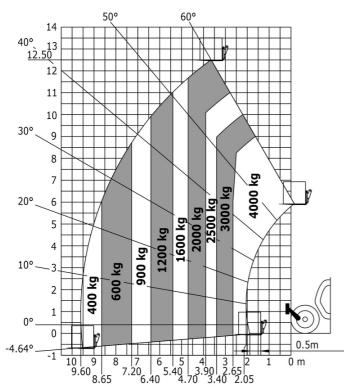
Machine on lowered stabilisers with forks Metric
