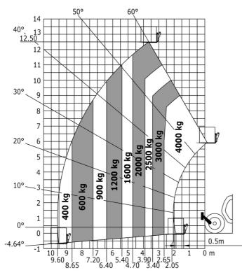
Machine on lowered stabilisers with forks Metric
