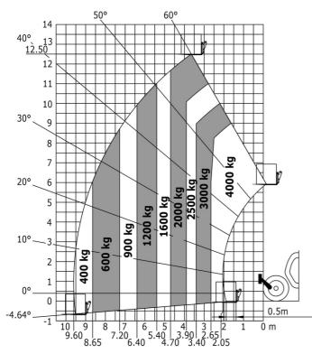
Machine on lowered stabilisers with forks Metric
