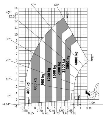
Machine on lowered stabilisers with forks Metric
