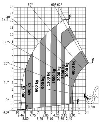
Machine on lowered stabilisers with forks Metric
