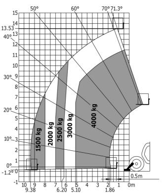
Machine on stabilisers with Man basket Metric
