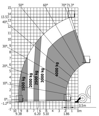
Machine on stabilisers with Man basket Metric
