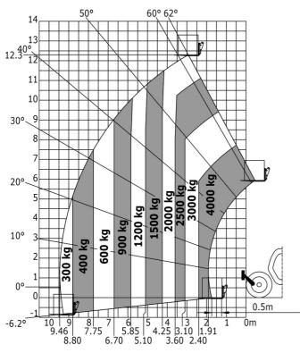
Machine on lowered stabilisers with forks Metric
