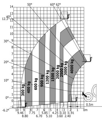
Machine on lowered stabilisers with forks Metric
