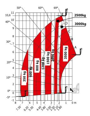
Machine on tires with forks - with levelling device Metric
