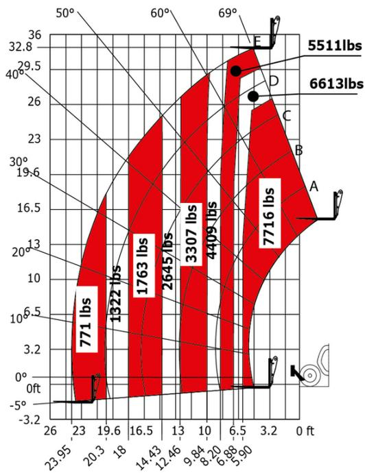
Machine on lowered stabilisers with forks Imperial
