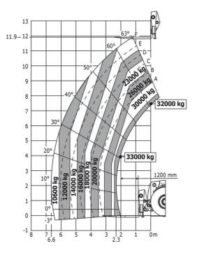
Machine on tires with 3-hook jib 36000 kg (Metric)
