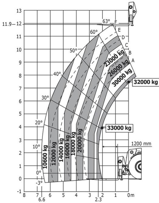
Machine on tires with hook 36000 kg (Metric)
