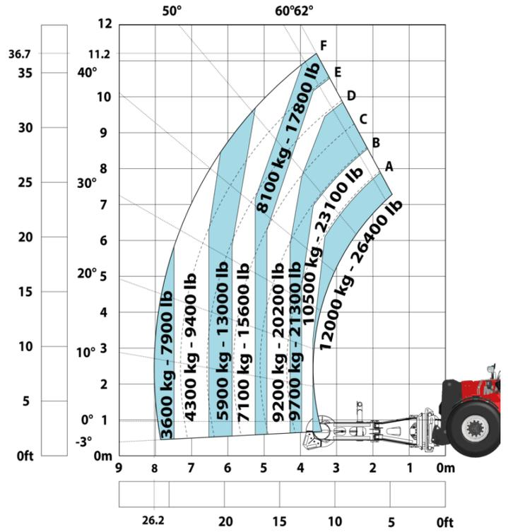
Machine on tires with cylinder handler CH 10 (Metric)
