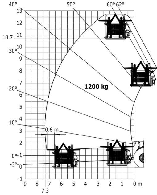
Machine on tyres with tyre handler TH 63 (Metric)
